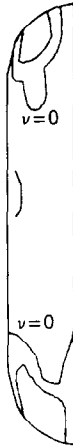
FIG. 6. Radial velocity contours in a vertical lamp ( \Delta v = 0.01 \text{ m s}^{-1} ).
